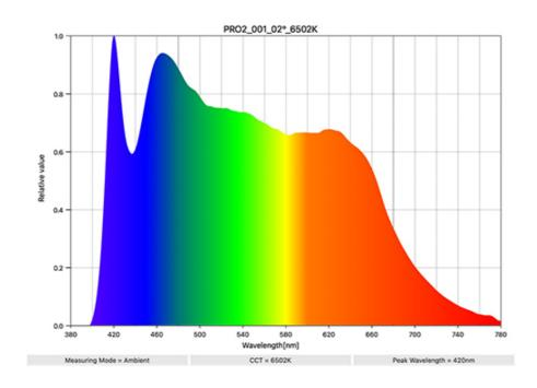
Most commodity LED lighting systems fall apart in the R9 value which is not included in CRI calculations, but is necessary for the faithful reproduction of skin tones and deep reds. They are often replaced with much more energy-efficient, and cheaper green phosphors, which can result in a greenish color cast, even when used to illuminate a grey surface, such as is the case with bias lighting.
