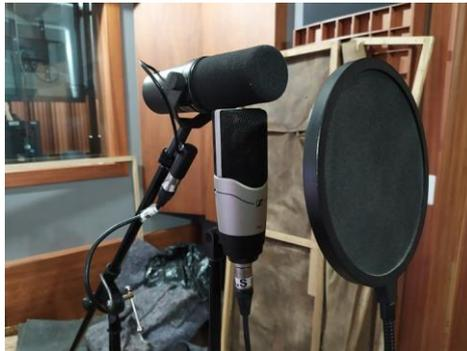
IMAGEN 14: MICRÓFONO SENNHEISER MK8 Y SHURE SM 7B
